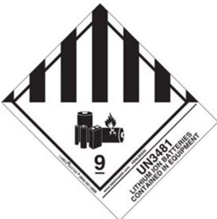
Class 9 Label (UN3481) "Contained In" Equipment
